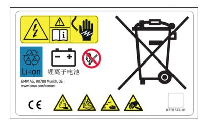
Example: "Li-ion" recycling symbol on the high-voltage battery
